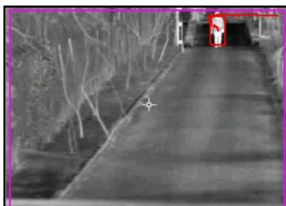
11. figure: Detecting and tracking a moving persons
