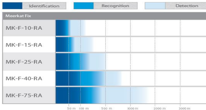
8. figure: DRI parameters of a few thermal cameras
