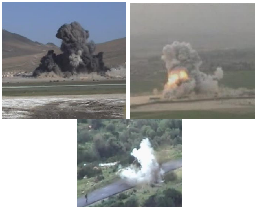
Fig. 10: Explosions with different smoke colours of TNT, ANFO and homemade charges
