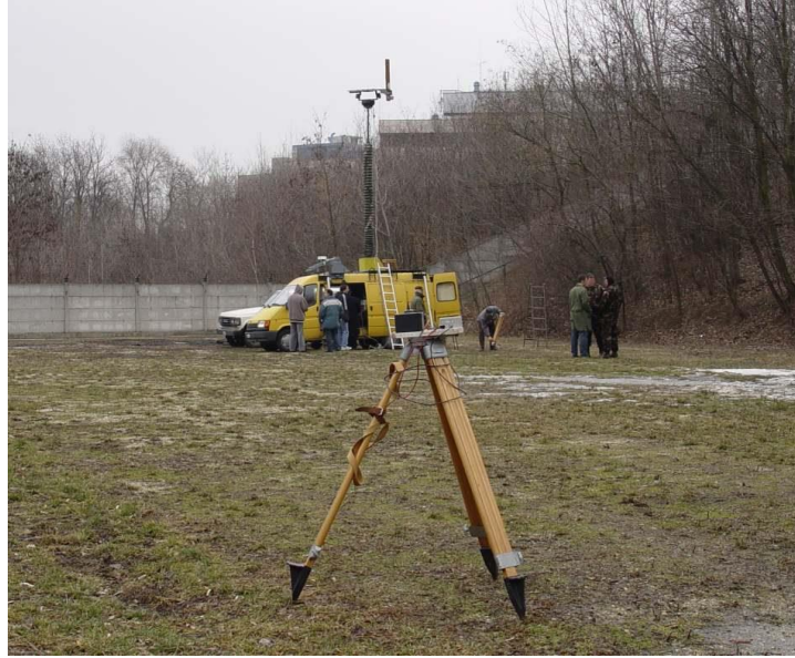
Photo 3. Measurement ( radio source in the foreground on a stand)
